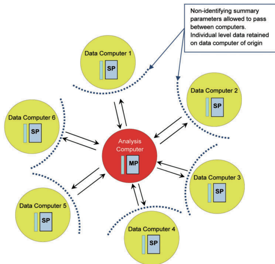
Figure 2 Schematic representation of the structure of DataSHIELD. The computer controlling analysis (heavily shaded circle) is sited at the analysis centre (MP: master process). The data computers (lightly shaded circles) are each sited at one of the study centres involved in the collaborative analysis (SP: slave process). The arrows indicate the flow of analytic instructions and summary statistics. All potentially disclosive individual-level data are secured on the local data computers
